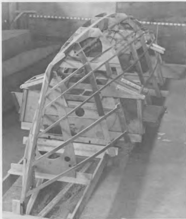
Trailertri 720 being built in Brazil by Jose Pedri and Jose Luz. Biggest problem is getting suitable metals.
