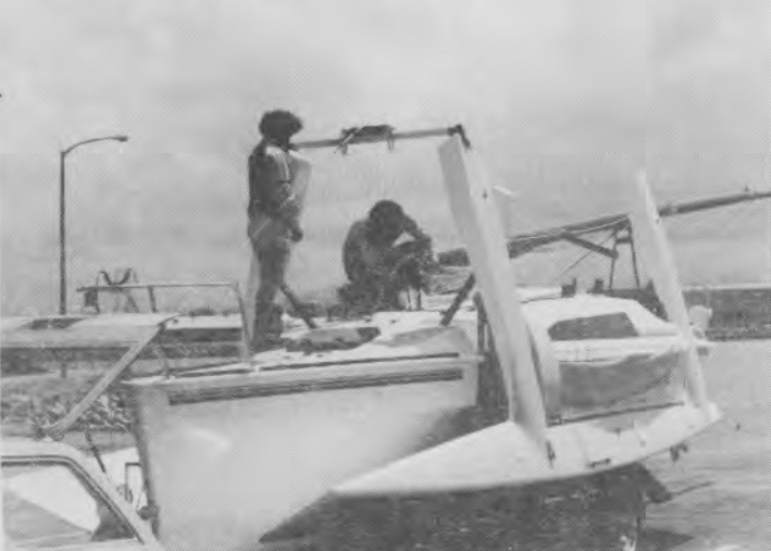
The mast is shown here ready for raising. The bar, with roller, on top of the forward beams makes this in one man job, in conjunction with the trailer winch.
