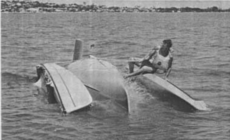
Folding while inverted was very simple. The righting ropes have already been fitted.
