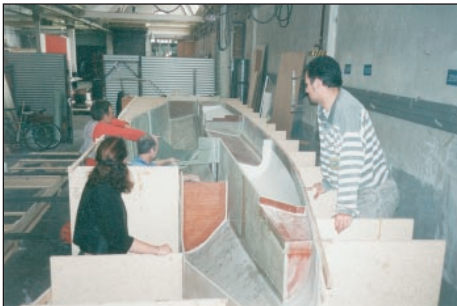
A stripped foam F-25A being built by Jurg Huber (now launched) in Switzerland, where there are now three F-25As, an F-25C, plus F-27s and F-31s. Building system with hull split vertically down center can be clearly seen - requires only half the form frames and saves a lot of time.
