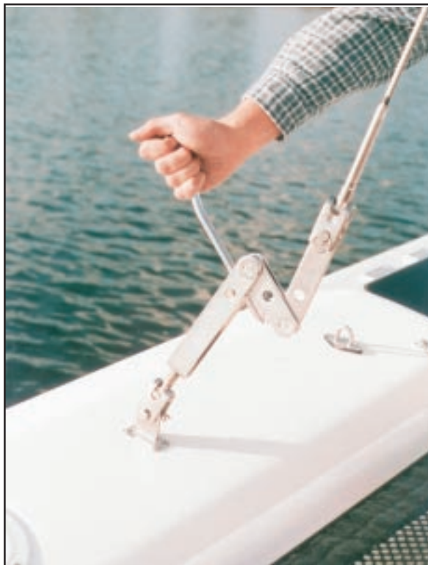
Highfield lever in operation - allows just enough slack for folding, and will still support mast when the boat is folded. Lever is locked by a center pin when closed.
