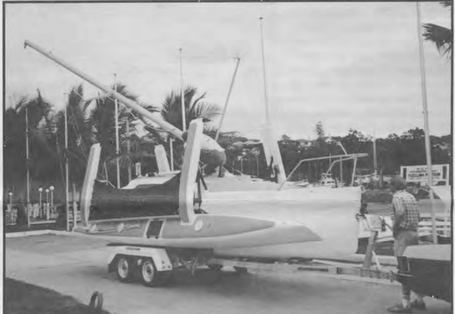
The first launching - 'plug in' mast raising pole being used to raise the mast. This system is now universally used on all F-Series designs and works very well, giving excellent leverage.
