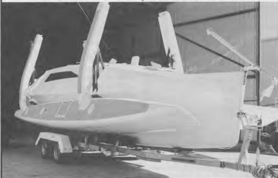
Custom built by Capricorn Hi Tech Yachts, Gladstone, by vacuum bagging over a male form. Was built for Denis Jobron, who is now taking it home with him to France.
