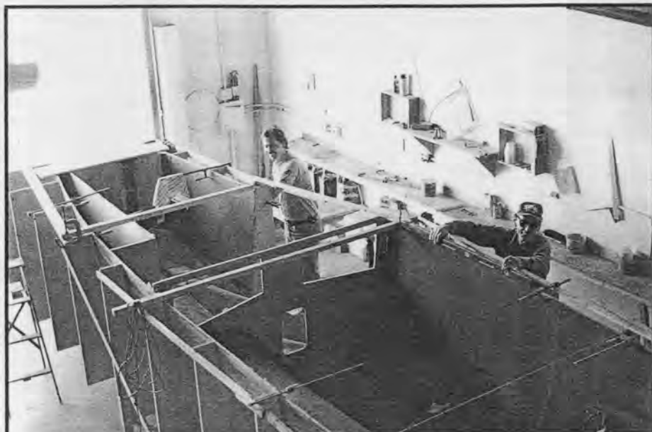
Steve Turansky's F-9A being built in Newport Beach, California. Hull half shown, black covering is carbon fiber.
