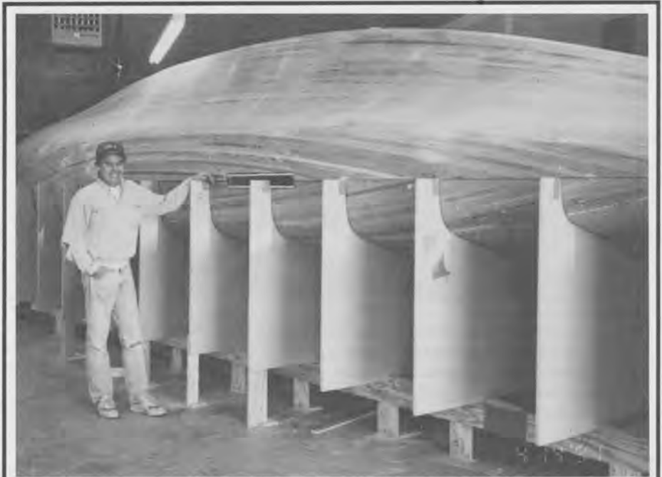
Mike and Pam Guthrie's new F-9A being built in Denver. Note the new method of building the main hull in two halves. This has proven to be a real time saver.
